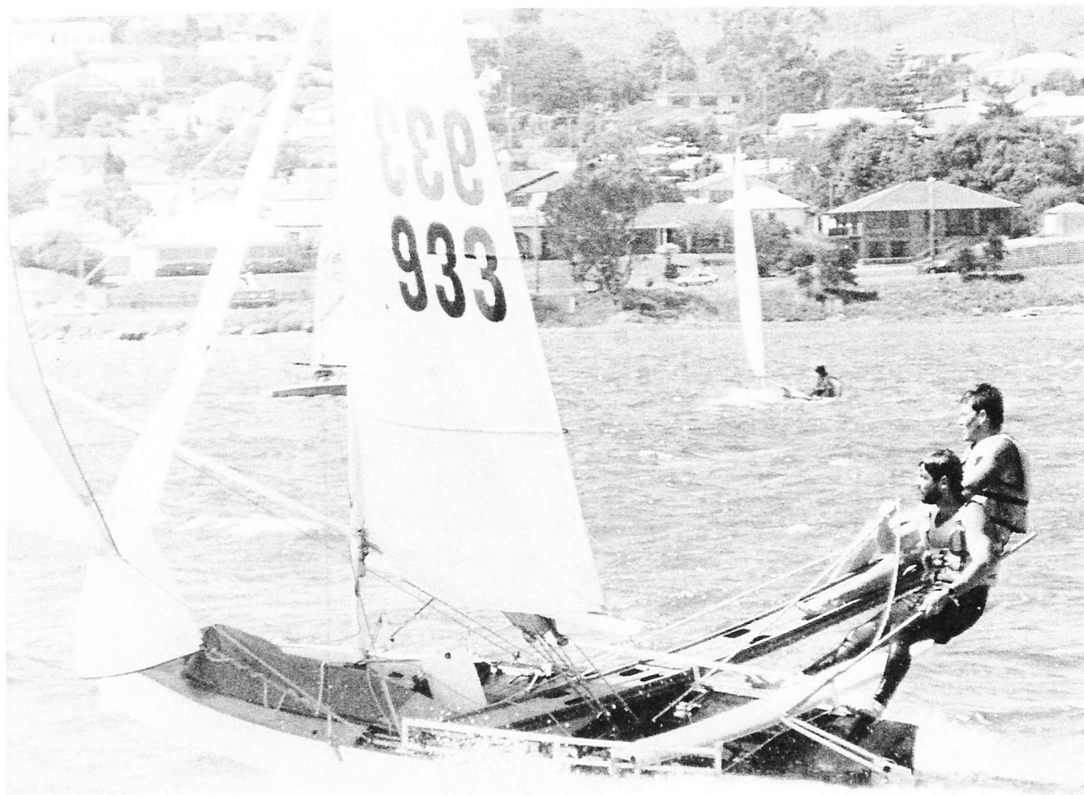
The 10 foot planks and big sail area make Skates powerful reaching boats.
